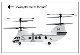
With the aileron stick pulled back, the 5-in-1 control unit alters the speeds of the front and rear rotors, causing the helicopter to move backward.
