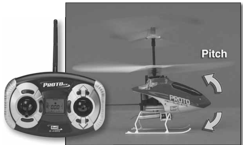
Moving the pitch/roll control stick forward and back controls the helicopter's pitch.
