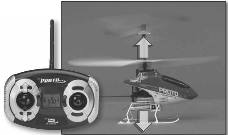
Moving the throttle/yaw control stick forward and back controls the helicopter's rotor blade speed which makes the helicopter climb or ascend.
