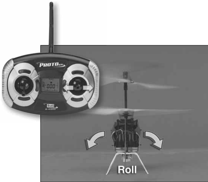
Moving the pitch/roll control stick to the left and right controls the helicopter's roll.
