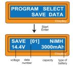
The parameter valaue setting up in this screen does not affect charge or discharge process. They only represent the specification of the battery. The following screens will automatically be displayed exactly matched with the
