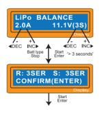
The value on the left side of second line sets a charge current and the value on the right side of second line sets the voltage of the battery pack.
