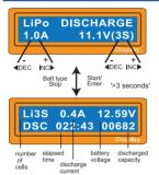
The value of discharge current on the left side of screen may not exceed 1C for a maximum safety and the final voltage on the right should not be under the voltage level that is recommended by the battery manufacturer to avoid deep discharging.
