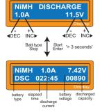
Set discharge current on the left and final voltage on the right. The discharge current ranges from 0.1 to 1.0A and the final voltage ranges from 0.1 to 25.0V). To start the process, press Start /Enter key more than 3 seconds
