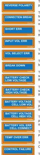
The output is connected to a battery with incorrect polarity.
