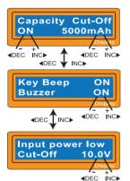
This program sets the maximum charge capacity that will be supplied to the battery during charge. If the delta-pack voltage is not detected nor the safety timer expired by any reason, this feature will automatically stop the process at the selected capacity value.
