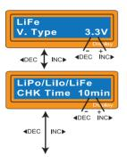
The screen displays the nominal voltage of Lithium battery. There are three kinds of Lithium battery; LiFe(3.3V),Lilo(3.6V) or LiPo(3.7V). This is very important so you have to check the battery carefully and set it up correctly. If it is different from correct value the battery can explode during charge process.
