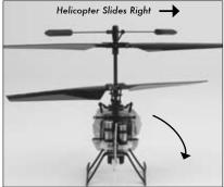
The aileron trim can be used to help keep the helicopter from drifting left or right when in hover with no aileron stick input. For example, if the helicopter drifts to the right when in hover, add left aileron trim until the helicopter hovers as level as possible with no drifting to the right.
