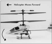
Pulling the stick backward will pitch the tail of the helicopter downward, allowing the helicopter to be flown backward.
