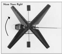
The rudder trim can be used to help keep the nose of the helicopter from rotating to the left or right when in hover with no rudder stick input. For example, if the nose of the helicopter drifts to the right when in hover, add left rudder trim (by pressing the left rudder trim button) until the nose stays as close to straight as possible.
