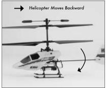
The elevator trim can be used to help keep the helicopter from drifting forward or backward when in hover with no elevator stick input. For example, if the helicopter drifts forward when in hover, add back/up elevator trim until the helicopter hovers as level as possible with no forward drifting.
