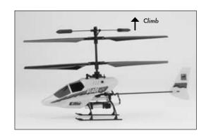
Decreasing the speed of the main rotor blades by lowering the throttle stick will cause the model to descend.
