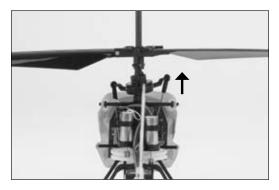
Move the right-hand stick left and right to check aileron roll control. When the stick is pushed to the left, the left-hand servo (when viewing the helicopter from behind) should pull the swashplate downward.
