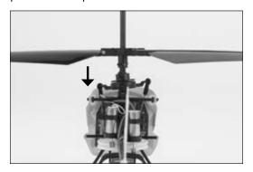
With the stick pushed right, the left-hand servo should push the swashplate upward.
