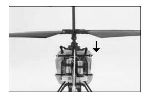
With the stick pulled back, the right-hand servo should push the swashplate upward.
